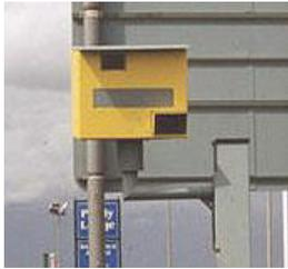
There are over 4,000 fixed Gatso speed cameras currently in use by police forces and local authorities across the UK, accounting for 90% of all fixed speed cameras. The Gatso which uses radar technology, is used for fixed speed cameras, in-car mobile units, on tripods and can even be used from moving vehicles.
