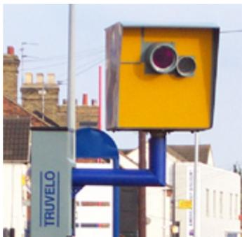
The forward facing Truvelo camera system is designed to take photographs of the front of a passing vehicle, this allows the picture taken to show the driver of the vehicle as well.
